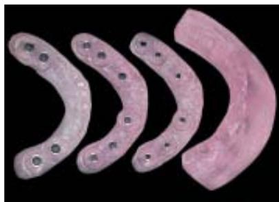
**Fig 1b** Materialise surgical guides and stereolithographic mandible fabricated from the virtual treatment plan.
